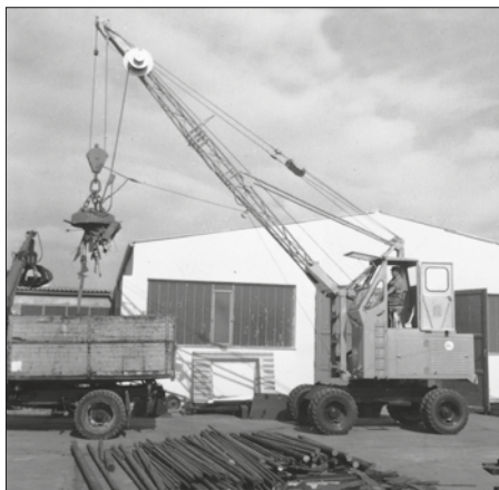
1962: rope-driven S833 with elevated operator cab
