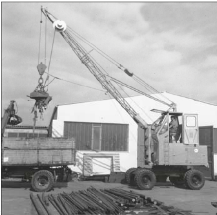
1962: rope-driven S833 with elevated operator cab
