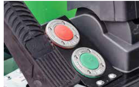
Comfortable pedals for continuous cab height adjustment
