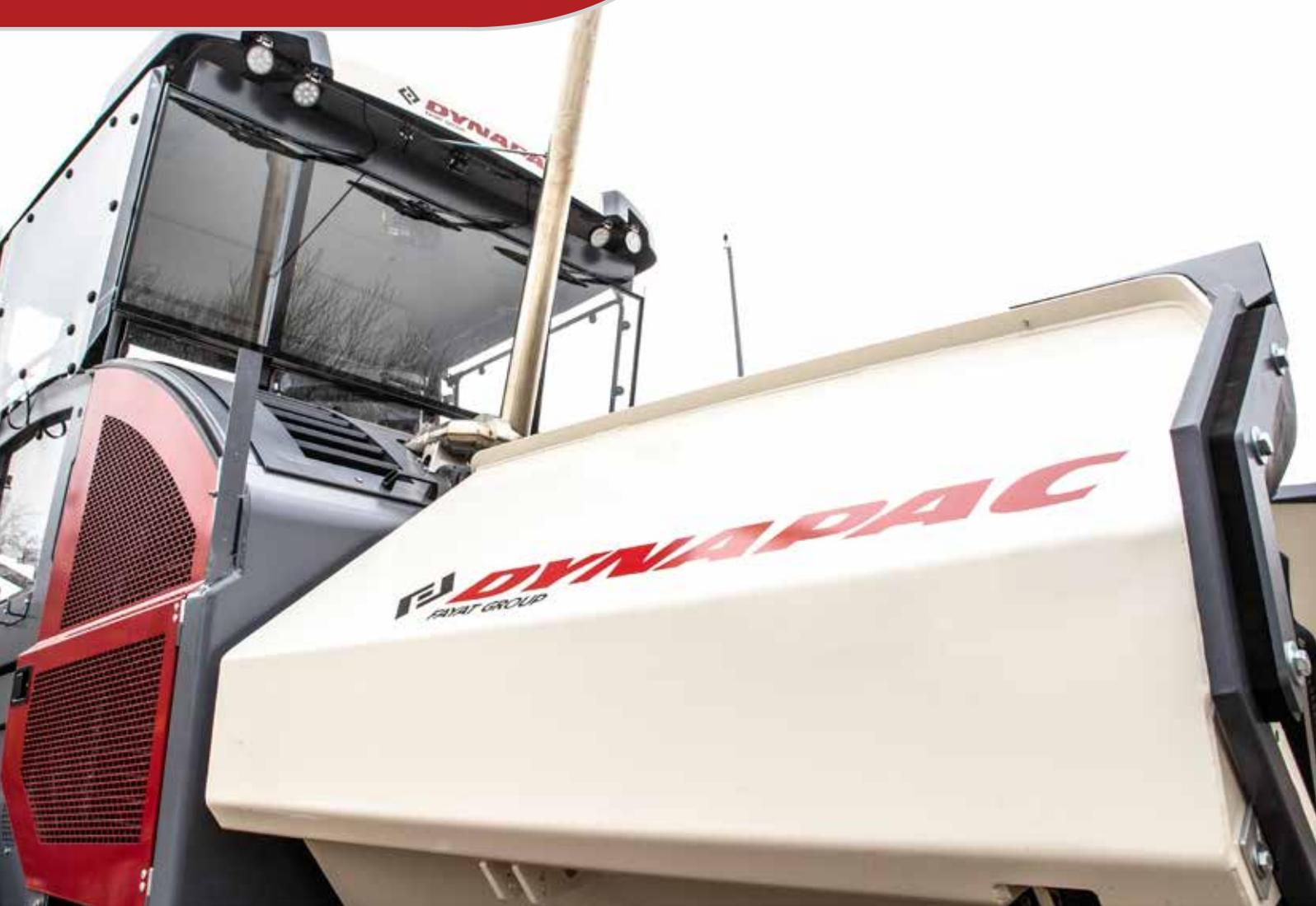
Dynapac SD Pavers are powered by a Cummins QSB6.7 diesel engine with emission Stage IIIA / IV & V. The power unit offers optimized energy conversion through: load-sensitive engine speed control; use of the most efficient pumps and the most compact final drives, incl. motors. The cooling system is driven by a hydraulic motor that is thermostatically controlled for efficient cooling. The CAN-BUS system ensures high operational reliability and centralised control.
