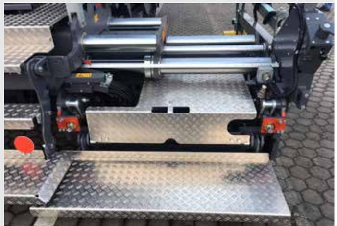
*There's no need for supporting rods for the screed, which makes all Dynapac screeds free floating – a must for excellent paving result!*
