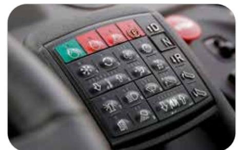
Keyless start, driver identity and access codes ensure no unauthorised operation of your equipment.
