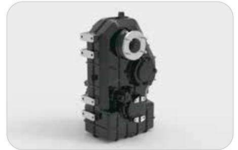
The transfer case inter-axle differential delivers equal torque to each axle when traction is favourable. When conditions deteriorate, the diff-lock automatically engages to deliver torque to the tyres that can best use it.
