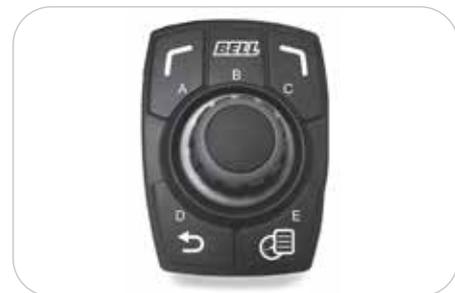
An automotive controller provides menu navigation on the colour monitor to extract information on machine operation and adjustment of machine settings.
