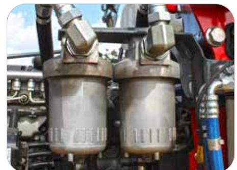
We offer a remote transmission filter option. They make transmission filter replacement a fast and clean task.
