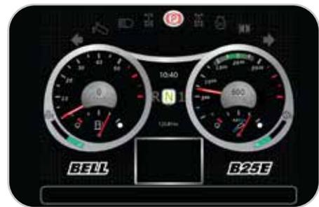
A user friendly 10" colour monitor offers vital operating information, safety warnings, detailed diagnostic readings and dump body function settings.
