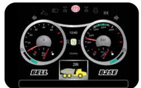
The exclusive on-board weighing presents the operator with real time information on the payload while the machine is being loaded. A 'speed restriction' mode can also be activated if the machine is significantly overloaded.
